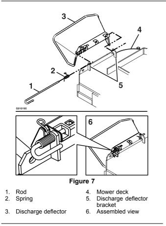
3. Hook the bent end of the rod around the front discharge deflector bracket to retain it from sliding out. Place the leg of the spring with the loop in the notch in the discharge deflector to hold the discharge deflector in the down position (see Figure 7).
